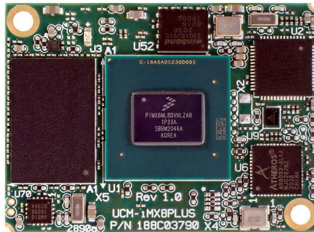
**UCM-iMX8M-Plus is an ultra-miniature Computer-on-Module (CoM) that features high performance graphics and imaging capabilities as well as impressive power efficiency. Ideal for a wide range of space constrained applications such as wearable healthcare monitors, medical devices, portable handheld devices and instrumentation equipment.**
